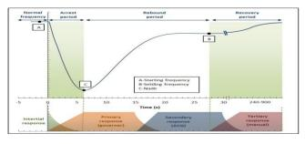
The second phase which has begun with the AGC automatic deployment is followed by secondary response (manually deployment of reserve) to return the frequency back to its nominal level. Finally, the slower Tertiary response, which are mostly off-line generation recalled in commission, replace the first and Secondary resources and reestablish the facility system ability to counter another contingency.
