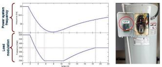
Frequency variation and load modulation for a Soft-R3 installed on a domestic water heater
